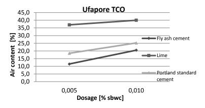
Mortar tests are performed according to EN 1015 in a standard mix without any other additive than air entrainer.
